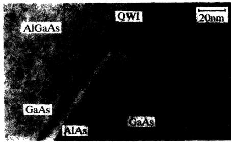
FIG. 1. Cross-sectional TEM micrograph of the top part of the facet structures. GaAs (black) ridge quantum wires 9 nm thick and 18 nm wide are formed between  $Al_{0.3}Ga_{0.7}As$  (dark gray) and AlAs (bright gray) barriers.
