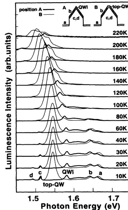
FIG. 2. PL spectra at various temperatures excited by He-Ne laser measured for the two regions, A (thick lines) and B (thin lines). The peaks are assigned as PL from ridge quantum wires (QWI), top quantum wells (top QW), bottom quantum wells (a), side quantum wells (b), and bulk GaAs (c, d).
