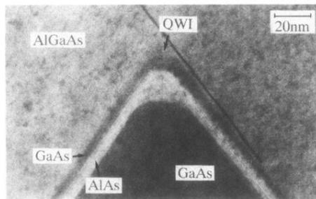
FIG. 1. Cross-sectional TEM micrograph of the top part of the facet structures. GaAs (black) ridge quantum wires 9 nm thick and 18 nm wide are formed between  $\text{Al}_{0.3}\text{Ga}_{0.7}\text{As}$  (dark gray) and AlAs (bright gray) barriers.
