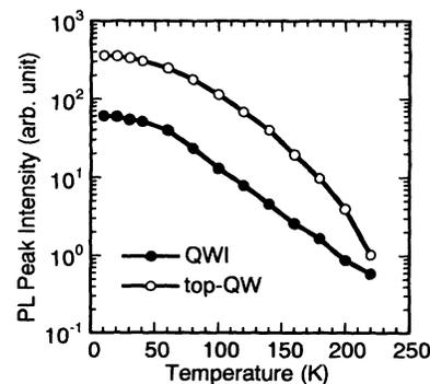
FIG. 3. Temperature dependence of PL peak intensities of QWIs and top QWs excited by He-Ne laser.
