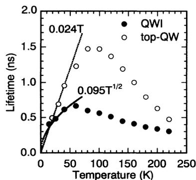
FIG. 4. Temperature dependence of PL decay time from ridge quantum wires (QWI) and top quantum wells (top QW) excited by the second harmonics of YLF laser pulses.
