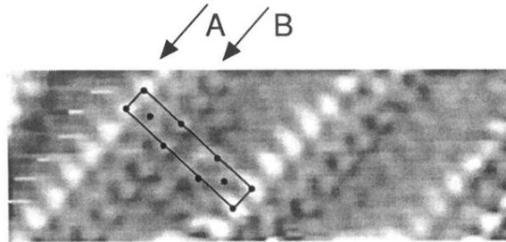
FIG. 2. The two-dimensional display of the image in Fig. 1(b). Superimposed on this image are the positions of "surface-layer" Ti atoms in the microfacet model of the  $1 \times 3$  unit cell [6]. The positions of atomically resolved features are indicated. The size of the image has been reduced by 16% to match the model.
