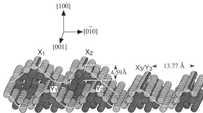
FIG. 4. A structural model of the intersection of [010]- and [001]-direction steps on vicinal  $\text{TiO}_2(100)-(1 \times 3)$  derived from the STM data. The relationship of the rows marked  $X_n$  and  $Y_n$  to the model are indicated. Small (large) spheres represent Ti (O) atoms, scaled to the appropriate ionic radii [9].
