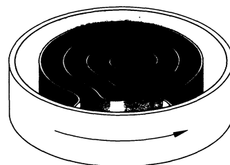
FIG. 1. Macroscopic structure of the vortex soliton in our cylindrical container rotating at \Omega = 0.58\text{ rad/s} . The structure is calculated assuming one sheet in contact with the wall, and following a local minimum of energy during increasing \Omega . The energy is approximated by the leading terms (isotropic kinetic energy and surface energy).
