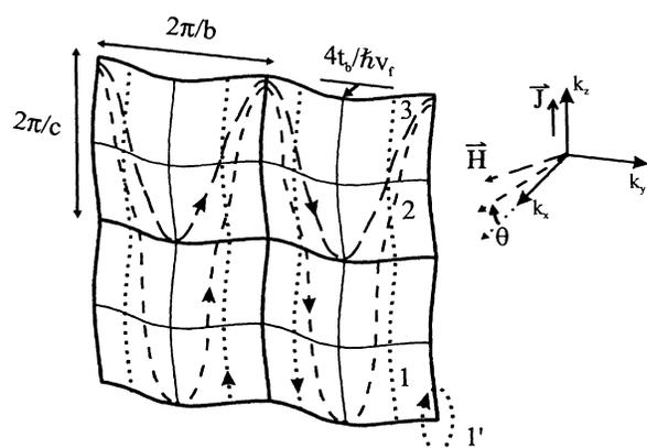
FIG. 2. The Fermi surface for  $(\text{TMTSF})_2\text{ClO}_4$ . Orbits 1 and 1' (dotted) show the approximate paths for electrons when the field is parallel to  $a$  for closed (1') and open (1) orbits. Orbits 3 (long dashed) and 2 (short dashed) show the paths when the angle of the magnetic field is near the primary maxima and the first secondary maxima of the data, respectively.
