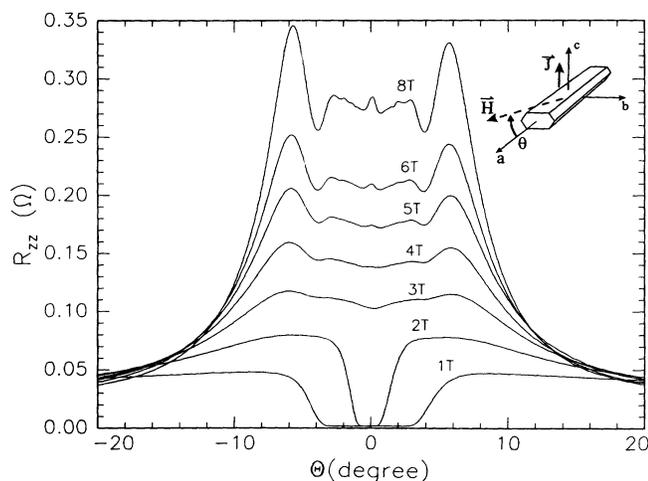
FIG. 1. Angular dependence of  $c$  axis resistance for rotations in the  $a$ - $c$  plane at different fields for  $(\text{TMTSF})_2\text{ClO}_4$  at  $T = 0.5$  K. The 2 T and 1 T traces exhibit superconductivity at smaller angles. Inset is a drawing of a crystal with axis, field, and current directions as shown.
