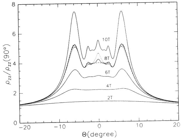
FIG. 3. Solid lines are the angular dependence of the calculated  $\rho_{zz}$  for different fields at fixed  $\tau = 4.3 \times 10^{-12}$  s. These curves use values of  $t_b = 0.012$  eV and  $t_c = t_b/15$ . The broken lines are for the same parameters as the 8 T solid line, except the dashed line uses  $t_c = t_b/7.5$  and the dotted line uses  $t_c = t_b/60$ .
