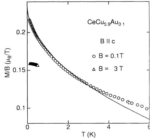
FIG. 2. Susceptibility  $\chi = M/B$  of  $\text{CeCu}_{5.9}\text{Au}_{0.1}$  in  $B=0.1$  T (applied to the easy direction) as a function of temperature  $T$  (circles). Solid line indicates a fit of  $\chi = \chi_0(1 - \alpha\sqrt{T})$  to the data. Also shown is  $M/B$  measured in  $B=3$  T (triangles).
