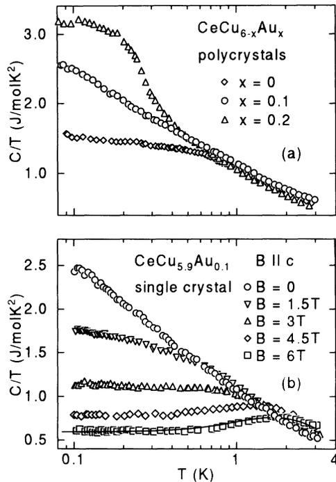
FIG. 1. (a) Specific heat  $C$  plotted as  $C/T$  vs temperature  $T$  (semilog) of  $\text{CeCu}_{6-x}\text{Au}_x$  polycrystals. (b)  $C/T$  vs  $T$  (semilog) for a  $\text{CeCu}_{5.9}\text{Au}_{0.1}$  single crystal for different magnetic field  $B$  applied to the easy direction. Solid line for  $B=6$  T indicates fit of the resonance-level model (see text).
