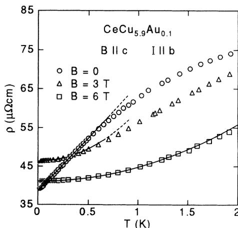
FIG. 3. Electrical resistivity  $\rho$  vs temperature  $T$  of  $\text{CeCu}_{5.9}\text{Au}_{0.1}$  for different magnetic fields  $B$  applied to the easy direction. Solid lines indicate fits with a  $T$ -linear ( $B=0$ ) and  $T^2$  dependence ( $B=3$  and  $6$  T).
