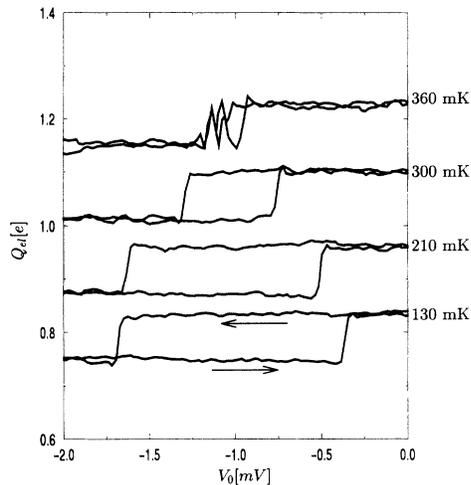
FIG. 2. Electrometer's charge vs applied trap voltage at (a)  $T = 0.130$  K, (b)  $T = 0.21$  K, (c)  $T = 0.30$  K, (d)  $T = 0.36$  K.  $V_0$  is ramped at a speed of  $0.3$  mV/s. The arrows indicate the direction of the voltage sweep. The curves are vertically offset for clarity.
