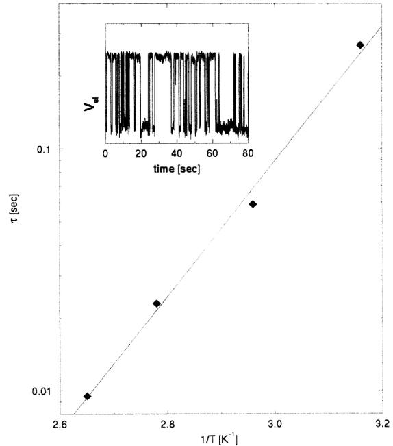
FIG. 3. Arrhenius plot of measured lifetime vs temperature. The slope of this plot gives the thermal activation energy  $E_a = 6.4 \pm 0.3$  K and  $\ln(\text{prefactor}) = -21.7 \pm 1.0$ . The inset is a time record of  $V_{el}$  at  $T = 0.32$  K.
