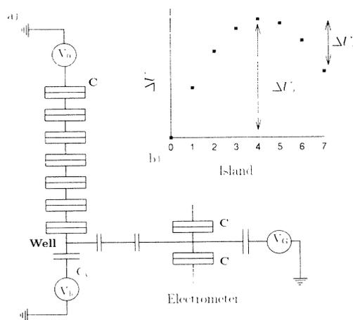
FIG. 1. (a) The schematic of a single electron trap and its monitoring SET electrometer. (b) The energy configuration diagram showing the change in free energy,  $\Delta U$ , associated with placing an electron on a particular island.
