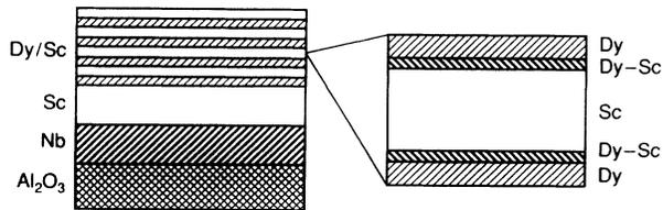
FIG. 3. Sketch of the Dy/Sc SLs, with the enlarged section to the right indicating the Dy-Sc alloyed layers on both sides of each Sc layers.
