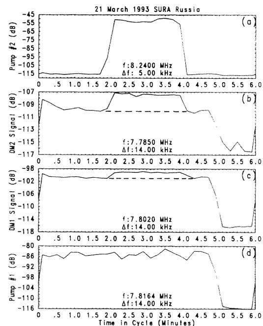
FIG. 2. Superposition of received powers for ten 6 min cycles of two frequency heating between 13:00 and 14:00 UT on 21 March 1993. Average powers for (a) pump 2, (b) DM2 of pump 1, (c) DM1 of pump 1, and (d) the carrier of pump 1 are obtained for the center frequencies ( $f$ ) and bandwidths ( $\Delta f$ ) shown. The average power for the downshifted spectrum from pump 1 is enhanced by 2 dB when pump 2 is transmitting.
