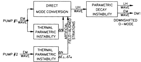
FIG. 3. Mechanism for the production of SEE with an intermediate upper hybrid (UH) wave. Two frequency electromagnetic (EM) wave interaction processes lead to enhanced downshifted maximum (DM1) emission. The addition of a second pump wave can enhance the mode conversion to upper hybrid waves by introducing additional field aligned striations.
