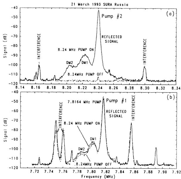
FIG. 1. Two frequency SEE spectra recorded together on 21 March 1993 between 12:00 UT and 12:04 UT at the SURA heating facility in Russia. The 8.2400 MHz electromagnetic pump 1 (a) is turned off (dashed line) for 2 min and on (solid) for 2 min while the 7.8164 MHz pump 2 (b) remains on for the 4 min interval. The downshifted spectral emissions (DM1 and DM2) for pump 1 are enhanced by 2 dB when pump 2 is turned on.
