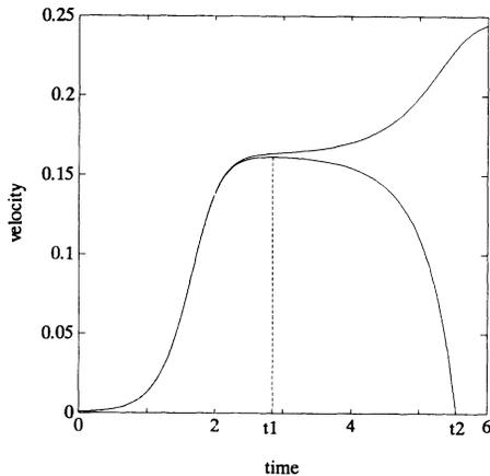
FIG. 1. Bubble velocities for two bubbles in a channel of length  $L=1$  with  $g=1$ . The initial conditions for the flow potential parameters are  $a_1=1.27e-6$ ,  $a_2=-6.35e-5$ , and  $a_3=0$ . The exponential rise, coexistence, and competition stages are clearly seen. For this bubble pair,  $q=1.03$  and  $\omega=0.37$ .
