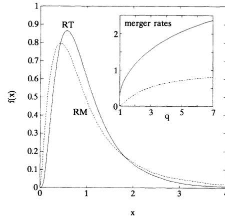
FIG. 2. Scale invariant bubble size distributions. The  $x$  axis is the bubble diameter in units of the average diameter. The full line is the result for RT fronts and the dashed line is for RM fronts. Inset: Dimensionless merger rates,  $\omega_0(q)$ , for the two instabilities. The upper line is for RT bubbles and the lower line is for RM bubbles.
