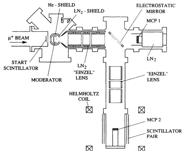
FIG. 1. UHV apparatus with cryostat used for the moderation studies. For details see text.
