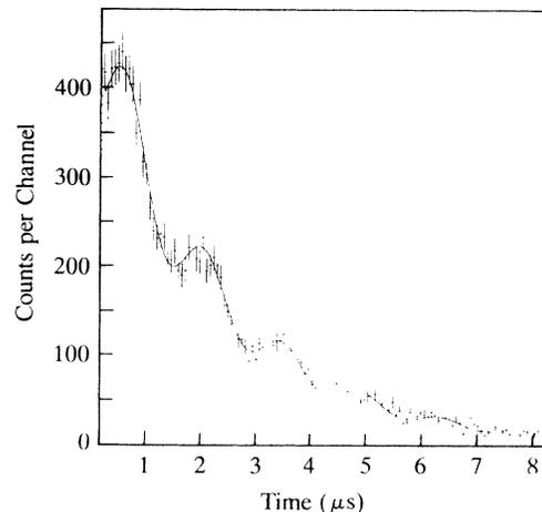
FIG. 3. Decay time distribution (left scintillator telescope) of the very slow  $\mu^+$  emitted from a solid Ar layer and precessing in a 50 G transverse magnetic field.
