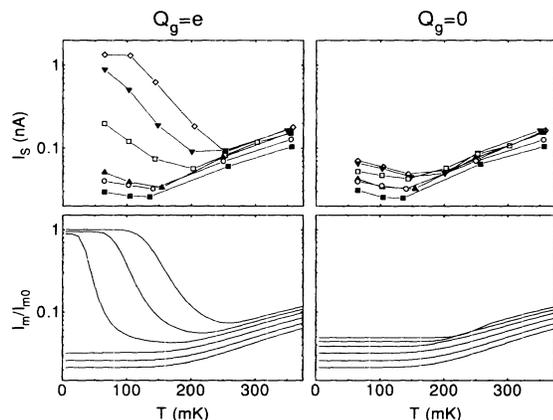
FIG. 5. Top panels: Experimental switching current as a function of temperature for  $Q_g=0$  and  $Q_g=e$ . Top to bottom, same field values as in Fig. 2. Bottom panels: Theoretical runaway current for the same conditions as in top panels. The theory curves reproduce the strongly nonmonotonous temperature dependence found in the experiment at  $Q_g=e$  for low fields.
