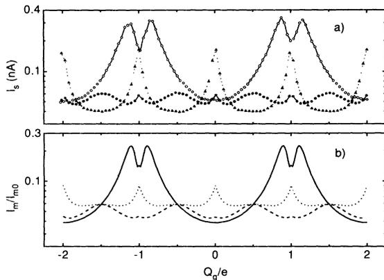
FIG. 4. (a) Switching current as a function of gate charge, at  $H=0.11$  T and for several values of the temperature  $T$ , showing the complex transition from  $2e$  periodicity to  $e$  periodicity with the increase of  $T$ . Open dots:  $T=65$  mK; solid dots:  $T=203$  mK; triangles:  $T=356$  mK. (b) Theoretical runaway current as a function of gate charge, for the same temperature values as in (a) (the full and dotted lines correspond to the lowest and highest temperatures, respectively).
