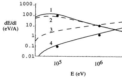
FIG. 1. The stopping of alpha particles by the ion component (curves 1 and 2) and the electron component (curves 3 and 4) of a  $10^{26} \text{ cm}^{-3}$ , 20 keV thermalized D-T plasma as predicted by Eq. (10) (solid circles), Eq. (11) (solid curves), and previous theory [3] (dashed curves).
