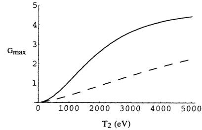
FIG. 2. The fusion energy multiplication factor for energy-clamped 100 keV deuterons within a  $5 \times 10^{13} \text{ cm}^{-3}$  thermalized tritium plasma. The evaluations shown use the stopping power as predicted by Eq. (11) (solid curve) and as predicted by previous stopping power theory [3] (dashed curve).
