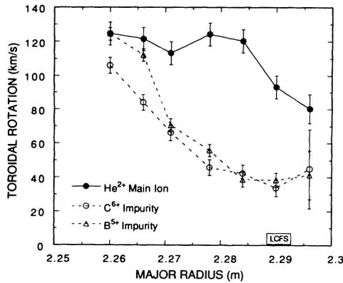
FIG. 2. Measured toroidal rotation of the main (helium) and the impurity (carbon and boron) ions in the edge region.
