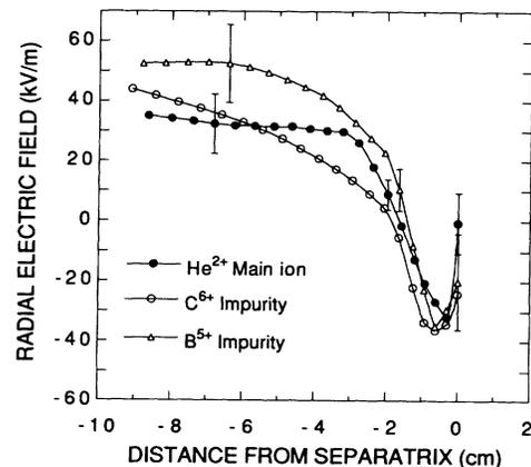
FIG. 4. Radial electric fields deduced from the main ion (helium) and the impurity ion (carbon and boron) measurements as a function of the distance relative to the LCFS.
