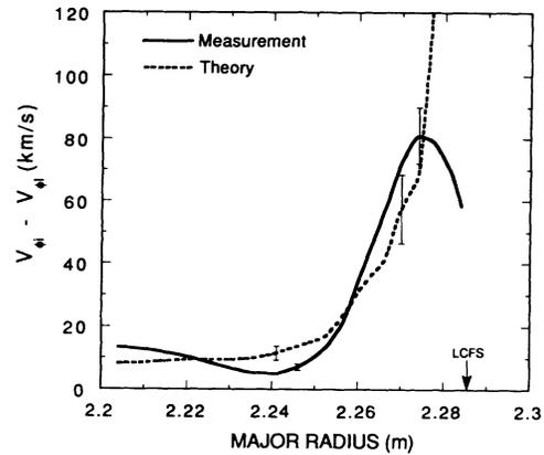
FIG. 3. Comparison of measured and predicted  $V_{\phi i} - V_{\theta i}$ , where two plasma shots (not exactly corresponding to the ones in Fig. 2) are combined ( $\text{He}^{2+}$  and  $\text{C}^{6+}$ ).
