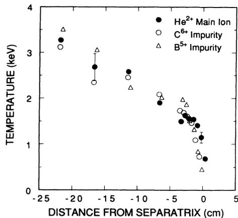
FIG. 5. Comparison of the temperature profiles obtained from  $\text{He}^{2+}$ ,  $\text{C}^{6+}$ , and  $\text{B}^{5+}$ .
