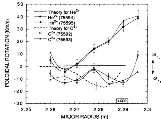
FIG. 1. Measured and calculated poloidal rotation of the main ions ( $\text{He}^{2+}$ ) and the impurity ions ( $\text{C}^{6+}$ ) in the edge region about 150 ms after  $L-H$  transition. The LCFS varies somewhat from shot to shot. The error bars represent 1 standard deviation of the random error.
