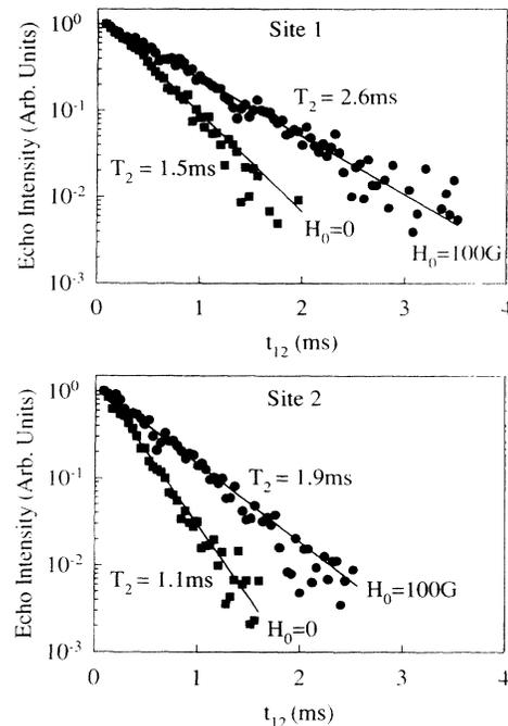
FIG. 1. Photon echo decays on the  $^7F_0 \rightarrow ^5D_0$  transition of  $\text{Eu}^{3+}:\text{Y}_2\text{SiO}_5$  at 1.4 K. The excitation density was  $6\text{ W/cm}^2$  and the straight lines are exponential fits to the decays yielding the dephasing times shown.
