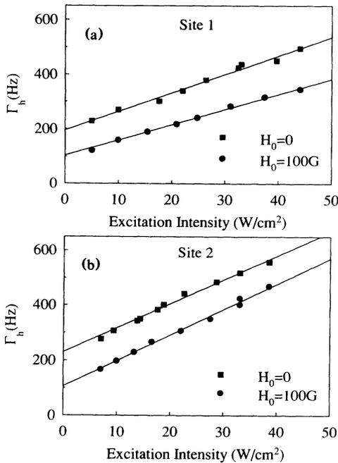
FIG. 2. Dependence of the homogeneous linewidth on excitation power density (a) for site 1 and (b) for site 2, varying both echo preparation pulses simultaneously. This shows the contribution from instantaneous diffusion. The linewidths extrapolated to zero laser power for  $H_0 = 100$  G are 105 Hz for both site 1 and site 2.
