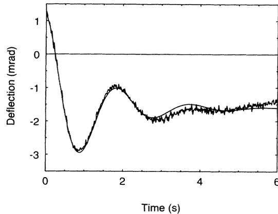
FIG. 4. Modulated response of the pendulum for 0.5 W microwave power incident on the pendulum without the linear thermal background. The theoretically predicted stationary deflection corresponding to  $1\hbar/\text{photon}$  is 1.7 mrad. The smooth curve is a least squares fit to the data.
