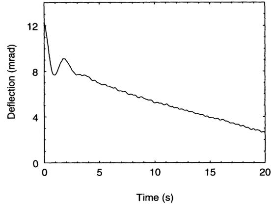
FIG. 3. Total response of the torsion pendulum for  $0.5 \text{ W}$  microwave power in a dielectric liquid illustrating the different time scales for thermal effects and effects due to transfer of photon angular momentum.
