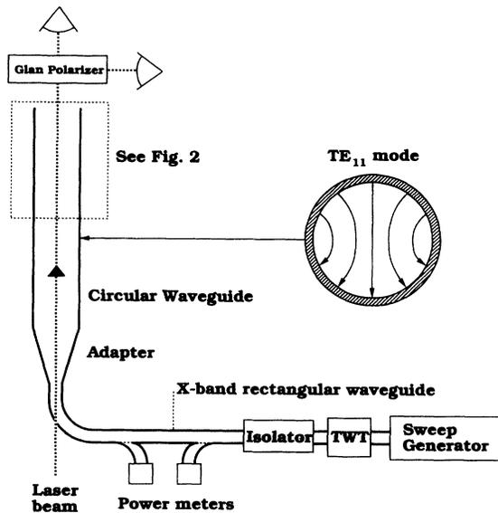
FIG. 1. Schematic diagram of the setup for measurement of the photon angular momentum in a dielectric material. The electric field pattern for the  $TE_{11}$  mode in the circular waveguide is inserted for illustration. The pattern rotates at the microwave frequency.
