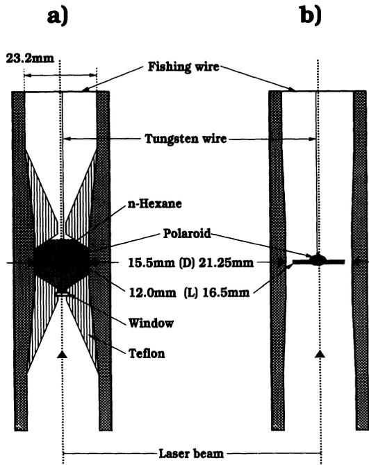
FIG. 2. Detailed view of the dipole antenna placed in the liquid (a) or in the empty waveguide with the same effective diameter (b). In both cases the antenna is suspended from a  $13.3 \mu\text{m}$  diam tungsten wire. The tungsten wire is attached to a piece of  $100 \mu\text{m}$  diam nylon fishing wire which spans the open end of the circular waveguide.
