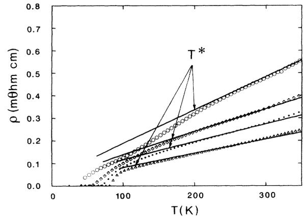
FIG. 2. Resistivity for  $\text{YBa}_2\text{Cu}_3\text{O}_{7-\delta}$  [11] compared with the theory, Eq. (14). For parameters see Table I.
