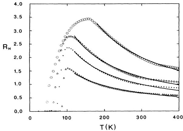
FIG. 1. Hall coefficient (in units of  $10^{-9} \text{ C}^{-1} \text{ m}^3$ ) for  $\text{YBa}_2\text{Cu}_3\text{O}_{7-\delta}$  [11] compared with the theory [Eq. (13), solid lines] for different  $\delta$ : 0.05 ( $\Delta$ ), 0.19 ( $\bullet$ ), 0.23 ( $\circ$ ), and 0.39 ( $\circ$ ). Parameters of the model are presented in Table I.
