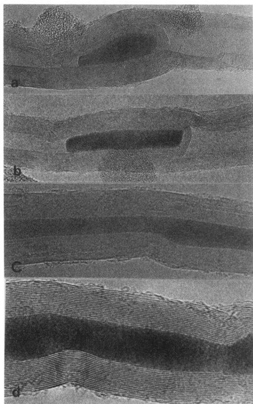
FIG. 2. (a),(b) High resolution images showing small precipitates of manganese trapped inside the fiber hollow and surrounded by graphite layers. (c),(d) Images showing the morphology of extended Mn fillings inside carbon nanofibers. Filling in (d) is slightly wavy but straight segments are seen in (c). Scale is 0.34 nm between the graphite basal planes (horizontal fringes) that make the fiber walls.
