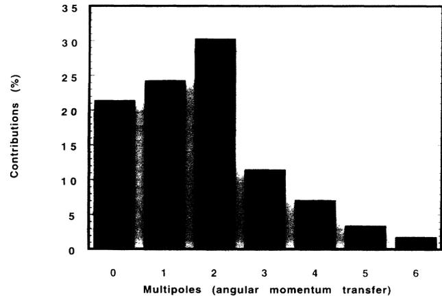
FIG. 3. Multipole contributions to the total cross section for double ionization of helium by Compton scattering at the photon energy of 12 keV.
