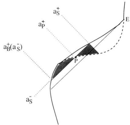
FIG. 2. The two shaded regions have equal area for any point  $(a_S^+, a_S^-)$  on the singularity curve.
