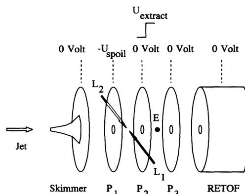
FIG. 1. Schematic of the experimental setup. See text for details.  $P_1$ ,  $P_2$ , and  $P_3$  are plates which have large diameters so as to exclude stray fields. The spoiling field is applied between  $P_1$  and  $P_2$  and the ionization/extraction pulse is applied (with a variable time delay) between  $P_2$  and  $P_3$ .  $L_1$  and  $L_2$  are the two lasers. The extraction of ions into the reflectron time of flight (RETOF) mass spectrometer occurs at  $E$ .
