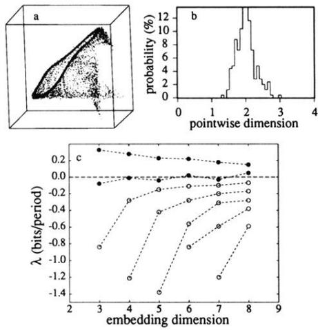
FIG. 4. Chaotic behavior in flash variation  $\Delta t$ . (a) is the attractor reconstructed from the flash time series. (b) is the distribution of pointwise dimensions for (a). (c) shows the results of calculation of the Lyapunov exponents for the attractor in (a).
