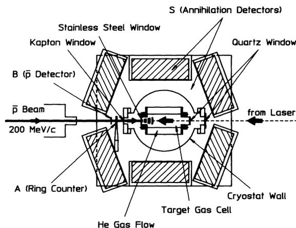
FIG. 2. Experimental setup. 200 MeV/c  $\bar{p}$ 's, passing through a beam counter ( $B$ ) and the hole in a ring counter ( $A$ ), are stopped in a target chamber containing helium, which is cooled to 5–10 K at 0.7–1 bar. Seven  $\bar{p}$  annihilation counters ( $S$ , 6 sides and 1 bottom) are located around the target. Two laser beams enter the target chamber through quartz windows from the direction opposite to the  $\bar{p}$  beam.
