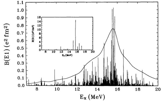
FIG. 1. Fine structure of the giant dipole resonance. The transition strength to each of the microscopically calculated states  $\Psi_\nu(\lambda\mu)$  is shown in histogram form. Also shown by the continuous curve is the transition strength obtained introducing an averaging parameter  $\eta = 500$  keV. In the inset, the transition strength obtained in RPA, neglecting the coupling with the two-phonon states, is displayed.
