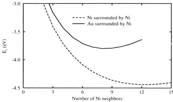
FIG. 3. The  $E_c$  function plotted as a function of coordination number  $N$  for a Ni atom and for a Au atom, in both cases surrounded by  $Ni$  neighbors at the equilibrium Ni bulk nearest-neighbor distance.
