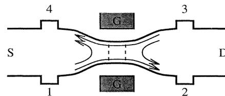
FIG. 1. Four-terminal Hall bar geometry with a narrow constriction between the source ( $S$ ) and drain ( $D$ ) formed by a lithographically patterned gate ( $G$ ). The dotted lines represent two parallel tunneling paths for quasiparticles. Precisely on resonance, there is perfect edge transmission between the source and the drain, as indicated by the arrows. Away from resonance the edge channels are reflected at low temperatures.
