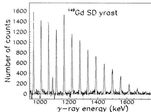
FIG. 1. Partial  $\gamma$ -ray spectrum corresponding to the yrast superdeformed band in  $^{149}\text{Gd}$  obtained by summing a number of combinations of three-dimensional energy windows set on fourfold coincidence events. A small fraction of the corresponding double-gated spectrum has been subtracted.
