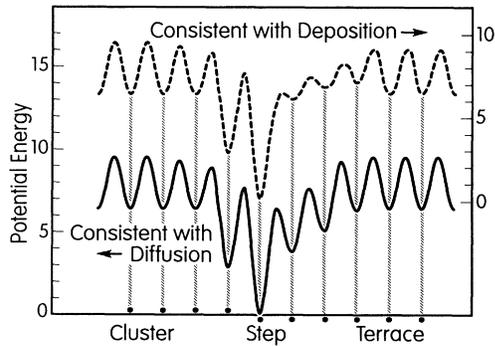
FIG. 5. Schematic of potential acting on adatom moving over a (111) plane with a central cluster. Bottom curve gives qualitative impression of potentials consistent with diffusion experiments [14]; curve at top suggests more severe alterations, which may account for atom behavior in condensation.
