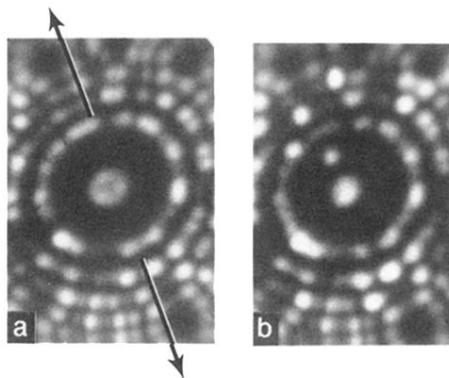
FIG. 1. Field ion image of Ir(111) with  $\text{Ir}_{12}$  cluster at the center. (a) Surface after formation of cluster by field evaporation. Arrows give projection of atom stream onto the (111) plane. (b) Same surface, after deposition of a single iridium atom onto the (111) plane at  $T \sim 20$  K.
