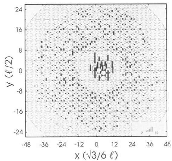
FIG. 2. Distribution of iridium atoms condensed on Ir(111) at  $T \sim 20$  K with central cluster of 12 iridium atoms on it. hcp binding sites are at intersections of grid lines. Height of bars indicates population on sites; calibration is given at lower right. The maximum plane diameter is  $26\ell$ .
