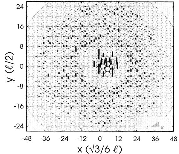
FIG. 2. Distribution of iridium atoms condensed on Ir(111) at  $T \sim 20$  K with central cluster of 12 iridium atoms on it. hcp binding sites are at intersections of grid lines. Height of bars indicates population on sites; calibration is given at lower right. The maximum plane diameter is  $26l$ .
