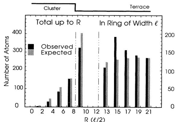
FIG. 4. Population of Ir atoms on Ir(111) with an  $\text{Ir}_{59}$  cluster at the center. Total number of atoms within a distance  $R$  from the center is plotted at left; shown at right is the population in a strip of width  $l$  at the indicated radius. Dashed lines indicate empty zone. The “expected” values are obtained on the assumption that atoms condense where they first land on the surface, except in the empty zone.  $l$  is the nearest-neighbor distance.
