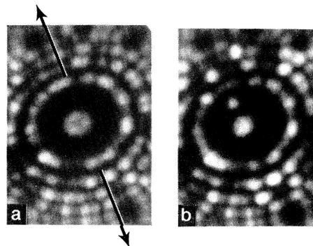
FIG. 1. Field ion image of Ir(111) with  $\text{Ir}_{12}$  cluster at the center. (a) Surface after formation of cluster by field evaporation. Arrows give projection of atom stream onto the (111) plane. (b) Same surface, after deposition of a single iridium atom onto the (111) plane at  $T\sim 20$  K.
