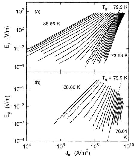
FIG. 2. Log-log plot of (a) the longitudinal electric field  $E_x$  and (b) the Hall electric field  $E_y$  vs the current density  $J_x$  at various temperatures and 3 T. Consecutive curves differ by temperature intervals of approximately 0.60 K. The dashed lines represent the power-law behavior at  $T_g$  (for  $E_x$  at "low" currents).
