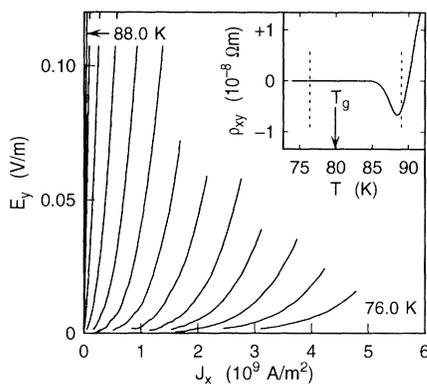
FIG. 1. Set of  $E_y$ - $J_x$  Hall curves at 3 T for temperatures between 76 and 88 K. Consecutive  $E_y$ - $J_x$  curves differ by temperature intervals of 1 K. The inset shows the linear Hall resistivity as measured at  $J_x = 5 \times 10^6$  A/m<sup>2</sup> and 3 T. The linear Hall effect changes sign around 90 K, and vanishes below about 83 K. The dashed lines delimit the temperature range in which the  $E_y$ - $J_x$  curves were measured.
