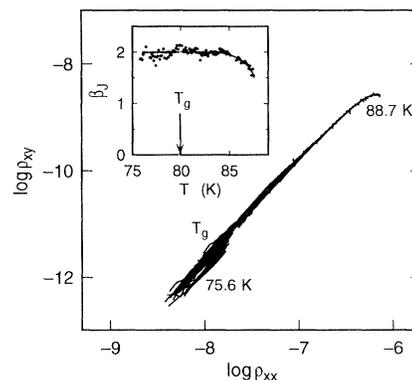
FIG. 4. Log-log plot of the Hall resistivity  $\rho_{xy}$  vs the longitudinal resistivity  $\rho_{xx}$  at 3 T. Both  $\rho_{xy}$  and  $\rho_{xx}$  are in units  $\Omega$  m. The curve is built up from over 100 isotherms, with  $J_x$  as running variable. These isotherms cover only part of the curve, as indicated by the labels. The inset shows the exponent  $\beta_J$  vs the temperature, demonstrating that Eq. (4) holds over a large range of temperatures.
