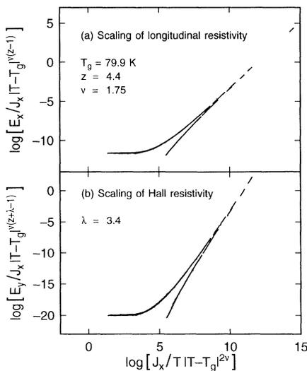
FIG. 3. Critical scaling collapse of over 100 isotherms between 76 and 86 K at 3 T for (a)  $E_x$  and (b)  $E_y$ .
