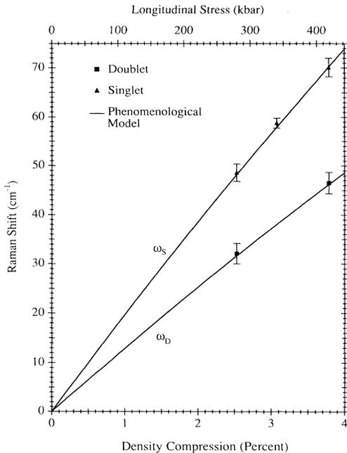
FIG. 6. Data from [100] compression experiments and comparison with phenomenological model predictions.
