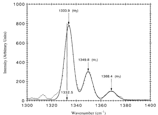
FIG. 3. Observed and fitted spectrum for [110] compression showing complete lifting of the triple degeneracy.
