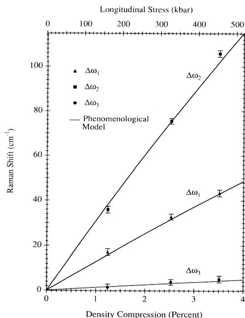
FIG. 4. Data from [110] compression experiments and fit to the phenomenological model predictions.
