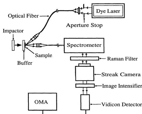
FIG. 1. Overall experimental configuration used for time-resolved Raman measurements in shock compressed diamond.
