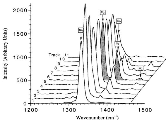
FIG. 2. Time-resolved, Raman spectra for [110] compression.
