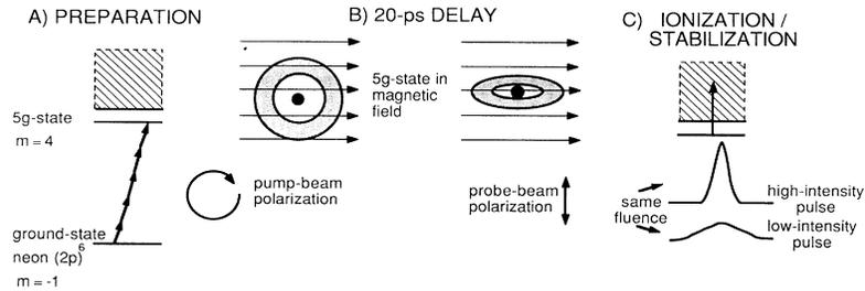
FIG. 1. Experimental scheme: (a) A pump pulse excites the  $5g$  circular ( $m=4$ ) state in neon. (b) We allow the atom to rotate due to a magnetic field (Larmor precession) until the atom is circular with respect to the vertical polarization of the probe laser. (c) Subsequently, the photoionization yield is measured using high- and low-intensity pulses of the same fluence.
