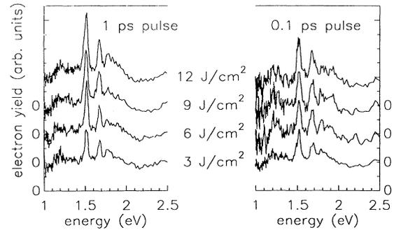
FIG. 3. Electron energy spectra for various fluences and two different pulse durations. The spectra are averaged over 2000 and 4000 shots for the long and short pulses, respectively. The background due to ionization when only the probe pulses are present has been subtracted. The peaks at 1.5 eV correspond to one-photon ionization of the  $5g$  state. For the short pulses the photoionization yields hardly increase with fluence.
