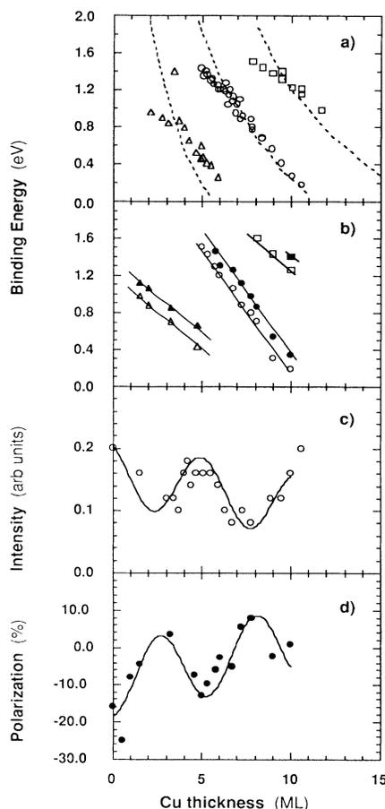
FIG. 3. (a) Binding energy of the features observed in the spin-integrated spectra (as in Fig. 1) as a function of the Cu overlayer thickness. (b) Binding energy of the features observed in the spin-resolved spectra (as in Fig. 2) as a function of the Cu overlayer thickness. (c) Spectral intensity at the Fermi level, after subtraction of the substrate contribution vs film thickness. (d) Spin polarization near the Fermi level vs film thickness.
