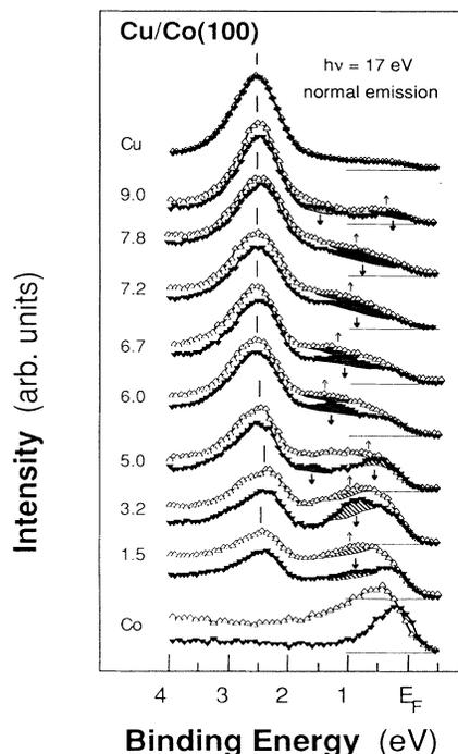
FIG. 2. Spin- and angle-resolved photoemission spectra of Cu overlayers on Co(100). The spectra are measured for normal emission with 17 eV photon energy. Open and closed triangles correspond to spin-up (majority) and spin-down (minority) electrons, respectively.
