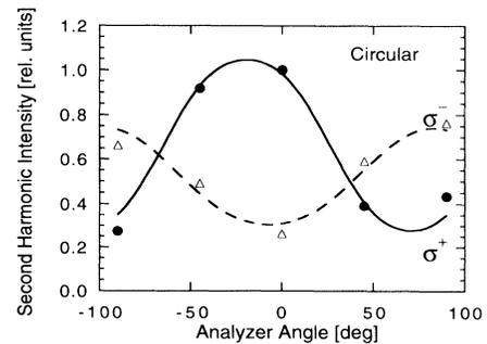
FIG. 2. Polarization analysis of SHG with circularly polarized incident light. The solid and dashed lines are fits to the data with  $\sigma^+$  and  $\sigma^-$  excitation, obtained by a convolution of the respective SH ellipse and the analyzer transmission [ellipticity:  $\epsilon^2(\sigma^+) = 0.987$  and  $\epsilon^2(\sigma^-) = 0.940$ ].
