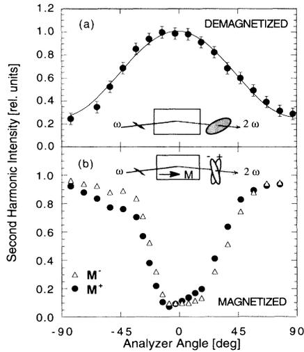
FIG. 3. Polarization analysis of SHG with  $p$ -polarized fundamental light. The analyzer angle is defined with regard to the plane of incidence. (a) Demagnetized sample; the solid line is a convolution of the SH ellipse and the analyzer transmission (ellipticity:  $\epsilon^2=0.981$ ). (b) Data from fully magnetized sample for opposite magnetization directions. The respective orientations of the SH polarization ellipse in the demagnetized and magnetized cases are illustrated in the two insets.
