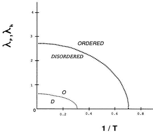
FIG. 1. The phase diagrams of the Lau-Dasgupta model (upper dashed line) and the model with close pairs only (lower dashed line). Simulations were carried out only along the axes. The ordered and disordered phases are marked for both models.
