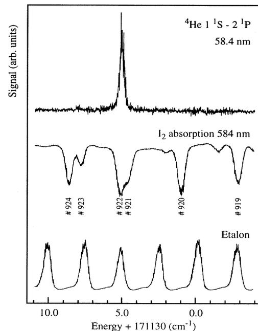
FIG. 2. The  $1^1S \rightarrow 2^1P$  resonance line of  $^4\text{He}$  at 58.4 nm recorded by 1 XUV+1 UV photoionization in the seeded beam. Also shown is part of an  $\text{I}_2$  absorption spectrum in the visible as well as a Fabry-Pérot spectrum. We used the lines labeled 920 and 924 in the iodine atlas [14] for calibration.
