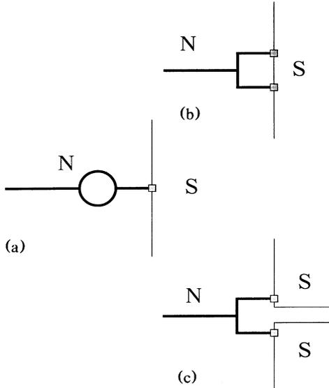
FIG. 1. Three geometries discussed in the text: (a) one-dimensional normal wire containing a loop connected to a superconducting electrode by a single junction; (b) fork geometry connected to the superconductor by two junctions; (c) fork geometry connected to two different superconductors.
