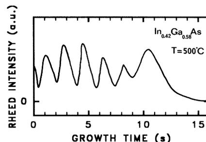
FIG. 1. Typical RHEED intensity oscillation observed during the growth of a highly strained InGaAs layer on GaAs (growth temperature 500°C). The growth is layer by layer (2D nucleation growth mode) up to 6 monolayers (ML), and then becomes highly 3D.
