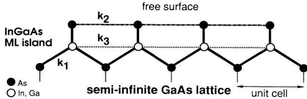
FIG. 4. Simplified model of interatomic forces in a 1D "island" of InGaAs on GaAs.  $k_1$  and  $k_2$  correspond to force constants for bond stretching while  $k_3$  is for bond bending.
