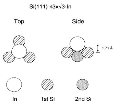
FIG. 2. Top and side views of the In/Si(111)- $\sqrt{3}\times\sqrt{3}$   $T_4$  geometry deduced from this work. The relative sizes of the In and Si atoms have been scaled to their covalent radii.
