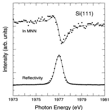
FIG. 1. Photon-energy dependence of the reflectivity and the background corrected In *MNN* x-ray standing wave near the Si(111) Bragg back-reflection condition for the In/Si(111)- $\sqrt{3}\times\sqrt{3}$  surface. The solid lines are the best fits to the data points (see text).
