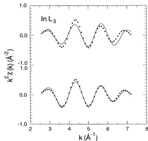
FIG. 4. Fits to the first-shell EXAFS data from the In/Si(111)- $\sqrt{3}\times\sqrt{3}$  surface assuming one (top) and two (bottom) first-neighbor bond lengths. The solid lines are the fits, and the dots are the data points of the backtransforms.
