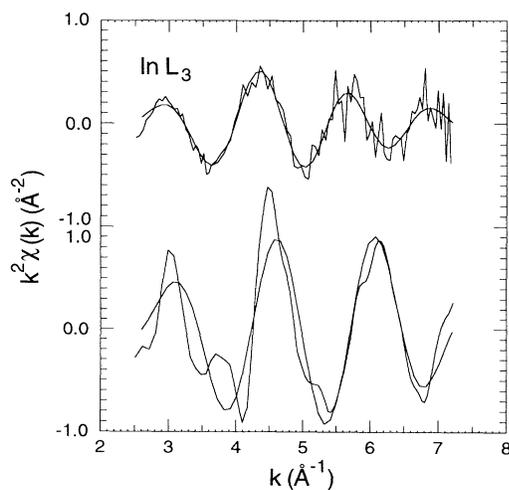
FIG. 3. Raw In  $L_3 k^2\chi(k)$  EXAFS data from the In/Si(111)- $\sqrt{3}\times\sqrt{3}$  surface (top) and from crystalline InP (bottom) plotted with their first-shell Fourier-filtered contributions.
