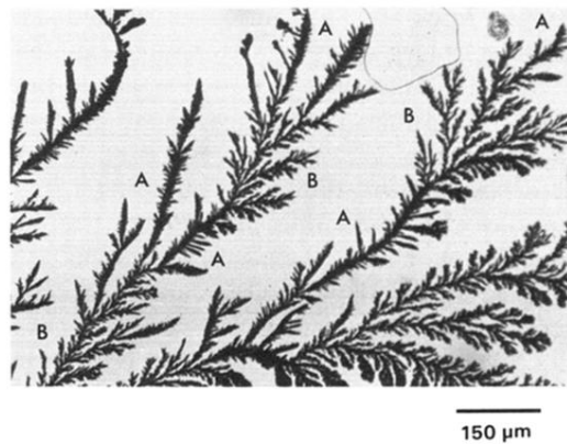
FIG. 1. The alternating morphology transitions observed in our system, in which dendrite and DBM regimes are labeled A and B , respectively. On the upper right corner of the figure, a hydrogen bubble hinders the dendrite growth.
