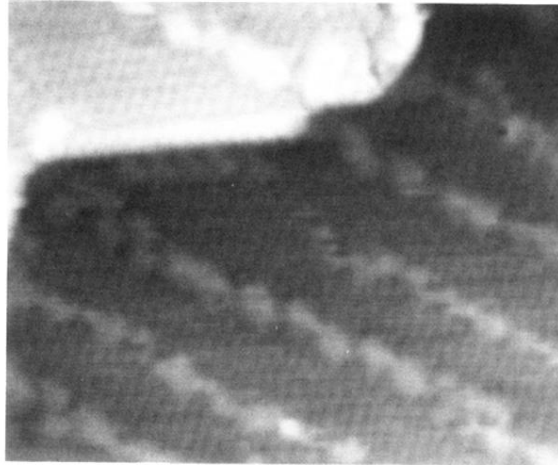
FIG. 5. Superstructure of site-exchanged ( 1 \times 1 ) domains. STM image after anneal to 1250 K. i_{\text{tunnel}} = 1 nA, V_{\text{sample}} = +1 V. Domain corrugation \approx 0.3 Å with walls \approx 0.6 Å tall.
