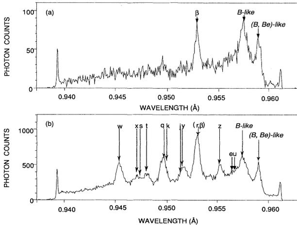
FIG. 4. Krypton  $K\alpha$  spectra measured by the TFTR vertical crystal spectrometer with a vertical sightline through the center of the vacuum vessel at  $R_0=2.65$  m. The data were accumulated (a) from 6 nearly identical Ohmic discharges with  $I_p=1.4$  MA, and (b) from 18 nearly identical Ohmic discharges with  $I_p=1.8$  MA.
