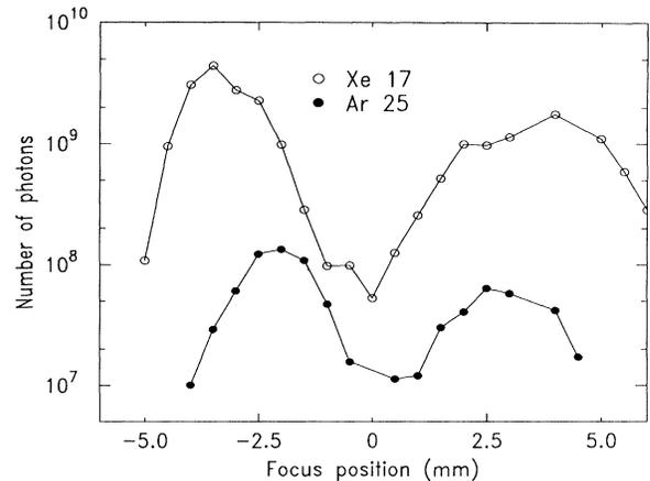
FIG. 4. 17th and 25th harmonics in Xe and Ar as a function of the position of the focus in the jet. The laser propagates from the left to the right.
