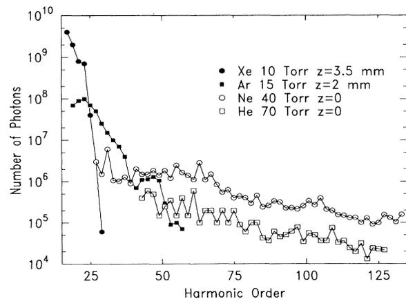
FIG. 3. Number of photons obtained per laser pulse in xenon, argon, neon, and helium as a function of the harmonic order.
