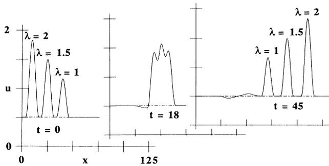
FIG. 1. The evolution of three  $K(2,2)$  compactons with speeds  $\lambda = 2, 1.5,$  and  $1$  starting with centers at  $x = 10, 15,$  and  $40$ .
