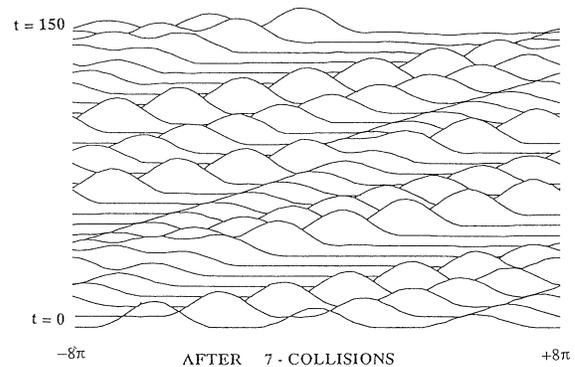
FIG. 2. Space-time plot of three compactons in Fig. 1 on a periodic domain. Note the phase shift whenever they collide.
