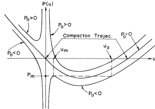
FIG. 5. Phase space of the three distinct classes of traveling waves in the  $K(2,2)$  equation; see Eq. (2b). For  $P_0 > 0$ ,  $u$  is either strictly positive or strictly negative. For  $P_0 < 0$ , depending on the value of  $P_1$ ,  $u$  is either strictly positive or changes its sign. Note that the local maximum at  $u = U_m$  gives rise to shelf solitons.  $P_0 = 0$  is a separating trajectory and describes trigonometric waves which turn into compactons when  $P_1 = 0$ .
