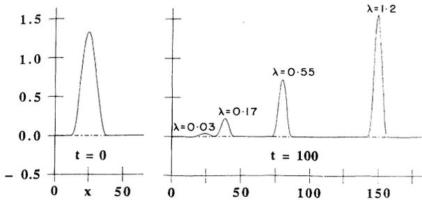
FIG. 4. The initial data  $u(x,t=0) = \frac{4}{3} \cos^2(x/2)$  decomposes into four compactons.
