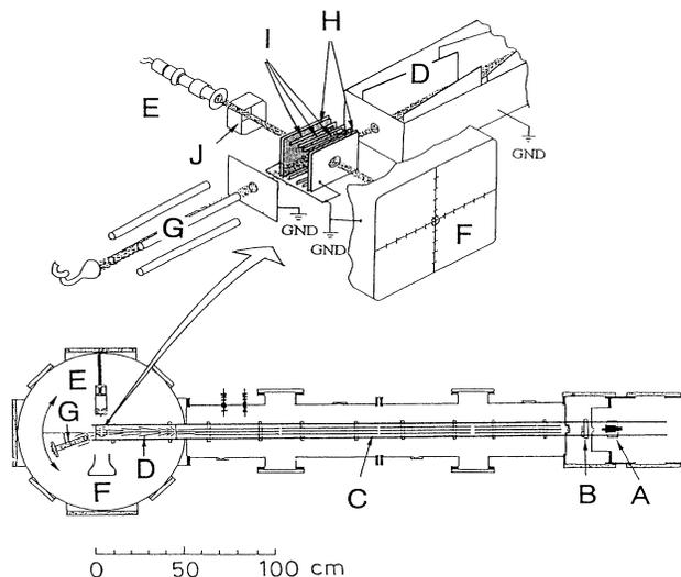
FIG. 1. Schematic view of the apparatus for electron impact with the oriented molecule. A, pulsed valve for  $\text{CH}_3\text{Cl}$ ; B, beam stop; C, electrostatic hexapole field; D, guiding field; E, electron gun; F, phosphorescent screen; G, quadrupole mass spectrometer; H, orienting field; I, field uniformers; J, electron beam deflectors.
