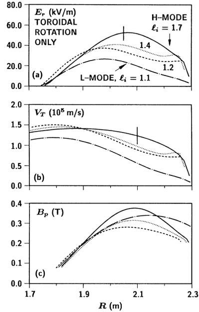
FIG. 4. (a)–(c) Comparison of  $V_T$ ,  $B_p$ , and  $E_R$  due to  $V_T$  across the midplane at 1950 ms (chain-dotted curves), 2500 ms (solid curves), 3200 ms (dotted curves), and 4000 ms (dashed curves) for a  $\kappa$  ramp discharge.
