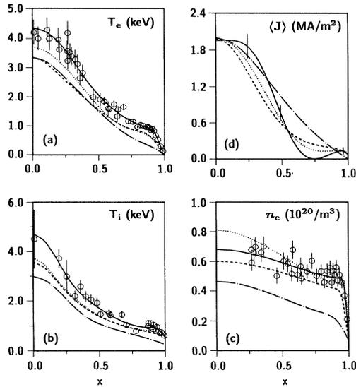
FIG. 3. (a)–(d) Comparison of  $T_e$ ,  $T_i$ ,  $n_e$ , and  $\langle J \rangle$  at the L-mode time 1950 ms (chain-dotted curves),  $l_i \sim 1.1$ ; and at the H-mode times 2500 ms (open circles and solid curves),  $l_i \sim 1.7$ ; 3200 ms (dotted curves),  $l_i \sim 1.4$ ; and 4000 ms (dashed curves),  $l_i \sim 1.2$  for a  $\kappa$  ramp discharge.
