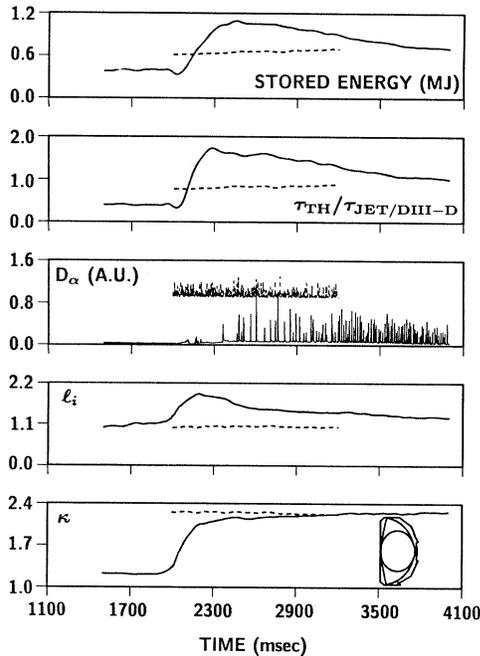
FIG. 1. Time evolution of  $W_T$ ,  $\tau_N$ , the line-averaged  $n_e$ , divertor  $D_\alpha$  radiation,  $l_i$ , and  $\kappa$  for a  $\kappa$  ramp discharge with  $P_{\text{NBI}}=5.7$  MW (solid traces) and a constant  $\kappa$  reference  $H$ -mode discharge with  $P_{\text{NBI}}=6.2$  MW (dotted traces). Also shown in the bottom panel are the poloidal cross sections from equilibrium analysis for the  $\kappa$  ramp discharge at 1950 ms and 2350 ms.
