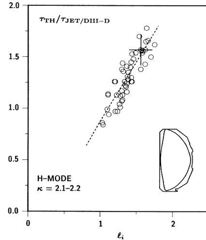
FIG. 2. Variation of the normalized thermal energy confinement time with  $l_i$ ,  $I_p=1-1.5$  MA,  $P_{\text{NBI}}=4-12$  MW,  $\tau_{\text{JET/DIII-D}}(s) \equiv 0.106 P_L^{-0.46} (MW) I_p^{0.03} (\text{MA}) R^{1.48} (\text{m})$  [8]. Also shown is the plasma poloidal cross section.
