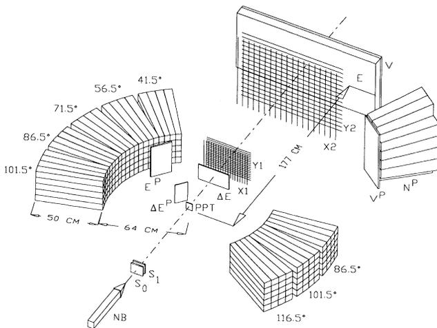
FIG. 1. Scale rendering of the experimental setup. Each stack of Pb-glass detectors is labeled by its central laboratory polar angle. Details are discussed in the text.
