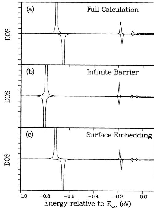
FIG. 2. Fe(110) spin-dependent density of states at  $\bar{\Gamma}$  integrated through the near-surface region (imaginary part of energy  $= 0.0001$  a.u.). The magnetic splitting found from the full calculations (a). The splitting caused by the spin-dependent surface barrier alone (b) and by the spin polarization of the substrate potential alone (c). Note how the splitting changes sign and becomes negative as the substrate magnetism is switched off.
