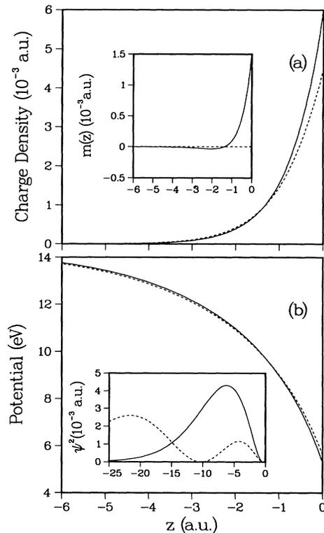
FIG. 4. Planar averaged electron density (a) and the interpolated surface potential (b) for spin up (solid line) and spin down (dashed line) directions in the near-surface region. The insets show the magnetization (a) and the probability densities of the first (solid line) and the second (dashed line) image state (b).
