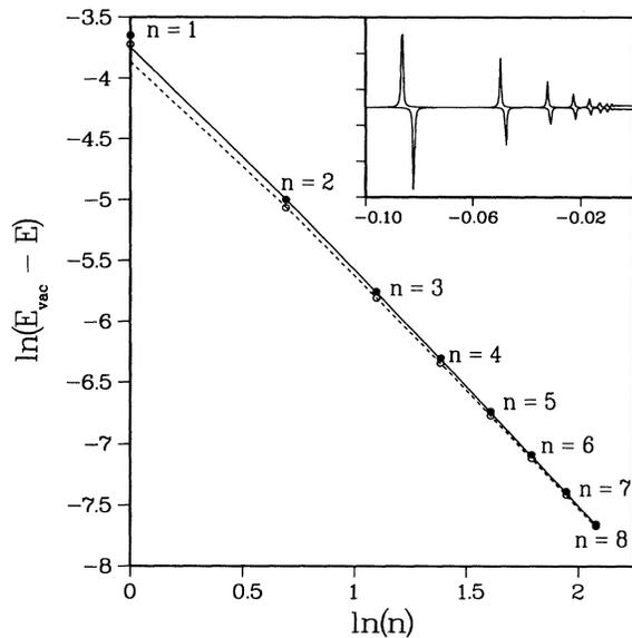
FIG. 3.  $\ln(E_n)$  vs  $\ln(n)$  for spin up (filled circles) and spin down (open circles) image states at the Fe(110) surface. The functions  $-\ln[32(n+a^{\dagger})^2]$  with  $a^{\dagger}=0.15$  (solid line) and  $a^{\dagger}=0.22$  (dashed line) are displayed for comparison. The inset shows the monotonic decrease of the spin splitting for  $n > 2$  members of the image series on Fe(110). These are resolved by working at a very small imaginary part of energy.
