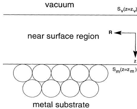
FIG. 1. Calculation geometry for the near-surface region embedded onto the metal substrate and vacuum. In the calculations  $z_m$  is located 2.35 a.u. above the last atomic plane. The near-surface region is 10 a.u. thick.
