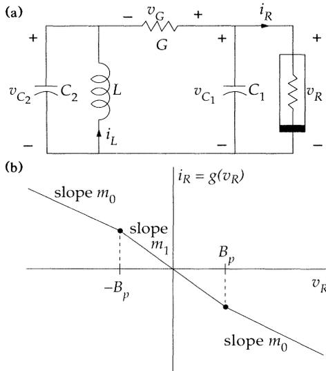
FIG. 1. Double scroll oscillator: (a) electrical schematic and (b) nonlinear negative-resistance  $i$ - $v$  characteristic  $g$ .
