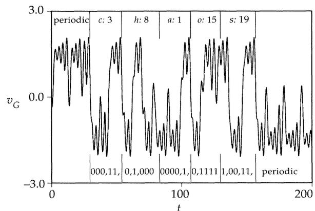
FIG. 4. Controlled  $v_G(t)$  signal for the double scroll system encoded with "chaos." Each letter is shown at the top of the figure, along with its numerical position in the alphabet. Shown at the bottom are the corresponding binary code words. Extra bits (indicated by commas) are added to satisfy the constraints imposed by the grammar.
