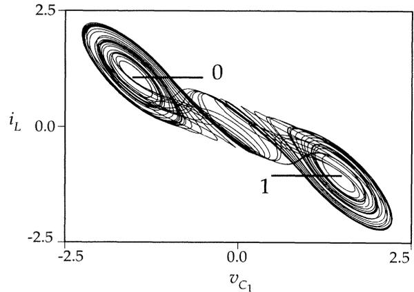
FIG. 2. Double scroll oscillator state-space trajectory projected on the  $i_L$ - $v_{C1}$  plane showing the two branches of the surface of section.
