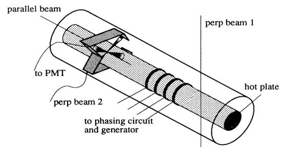
FIG. 1. The LMP experimental setup. The laser beams "perp 1" and "perp 2" are used to tag and detect test particles, respectively.
