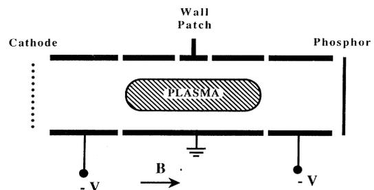
FIG. 1. Trap schematic.
