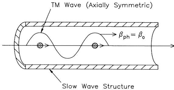
FIG. 1. Schematic of the beam conditioning configuration showing the axially symmetric, slow, TM wave conditioning properly phased electron pulses. The phase velocity of the TM wave is  $\beta_{ph}$  and the axial velocity of the reference electron is  $\beta_0$  (both normalized to the speed of light). An inductively generated electric field may be employed to cancel the accelerating component of the TM field.
